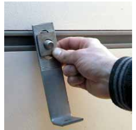
3. HALFEN T-bolts can be quickly be twisted into any position in the HALFEN channel. Nuts are simply tightened on HALFEN T-bolts to secure building components to the structure. Slotted brackets combined with HALFEN channels allow adjustment for accurate positioning in two or three dimensions.
