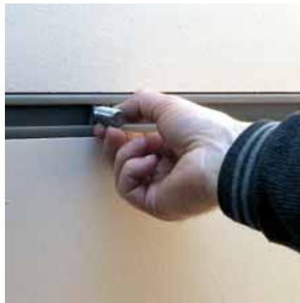
3. HALFEN T-bolts can be quickly be twisted into any position in the HALFEN channel. Nuts are simply tightened on HALFEN T-bolts to secure building components to the structure. Slotted brackets combined with HALFEN channels allow adjustment for accurate positioning in two or three dimensions.
