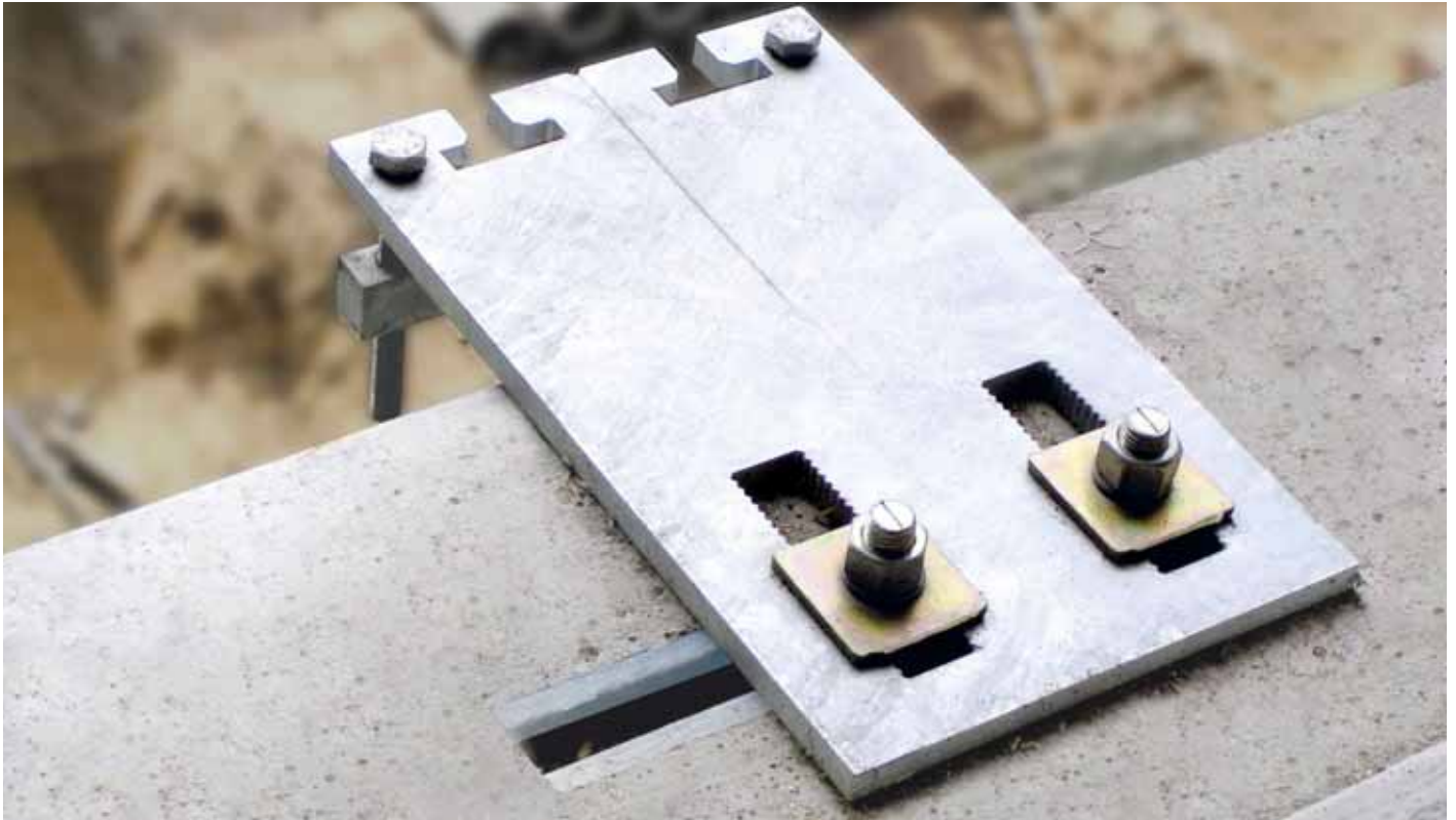
Curtain wall installation: Flush mounted HALFEN channels embedded in concrete mean that brackets can be pre-installed with the option of final adjustment when installing the façade panel.
