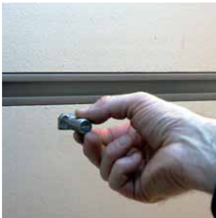
3. HALFEN T-bolts can be quickly be twisted into any position in the HALFEN channel. Nuts are simply tightened on HALFEN T-bolts to secure building components to the structure. Slotted brackets combined with HALFEN channels allow adjustment for accurate positioning in two or three dimensions.
