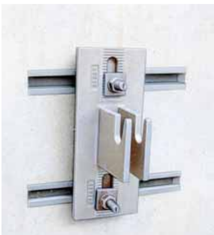
Façade installation: Pairs of HALFEN channels are suitable for transferring considerable tension and shear forces while providing easy installation adjustment
