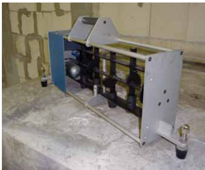
Standardised tapping machine according to DIN EN ISO 10140
