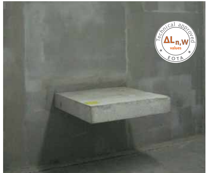
Test setup according to DIN EN ISO 10140 with built-in element
